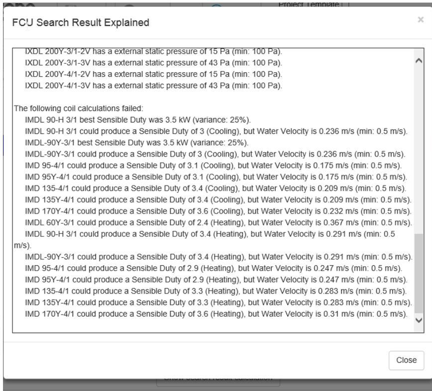
6. The same goes for the water velocity. Establish which of the cycles has the problem and try decreasing the LWT (Leaving Water Temperature) to reduce the water temperature split and therefore increase the flow and in turn the water velocity.
